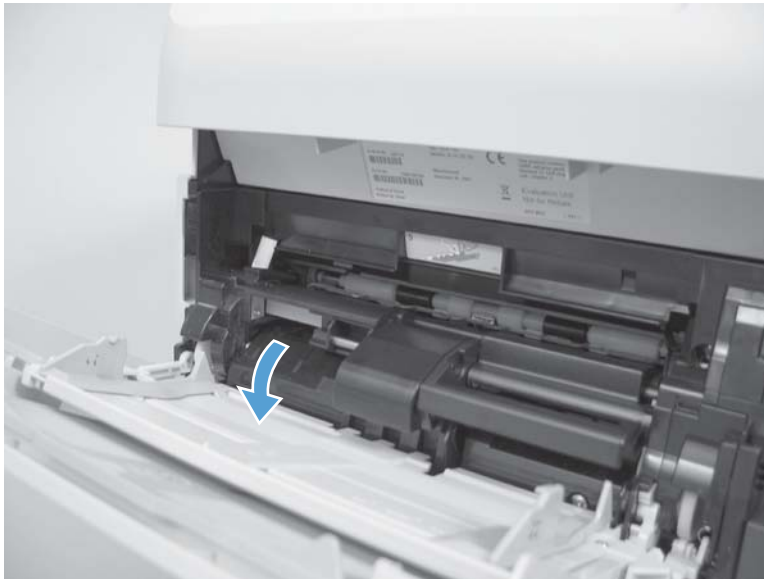
Figure 2-29 Remove the Tray 1 separation roller (1 of 3)
