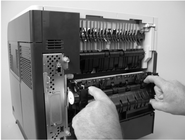
Figure 2-11 Remove the fuser (2 of 2)
