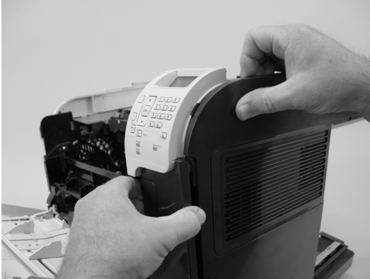
Figure 2-46 Remove the right-side cover (2 of 3)
