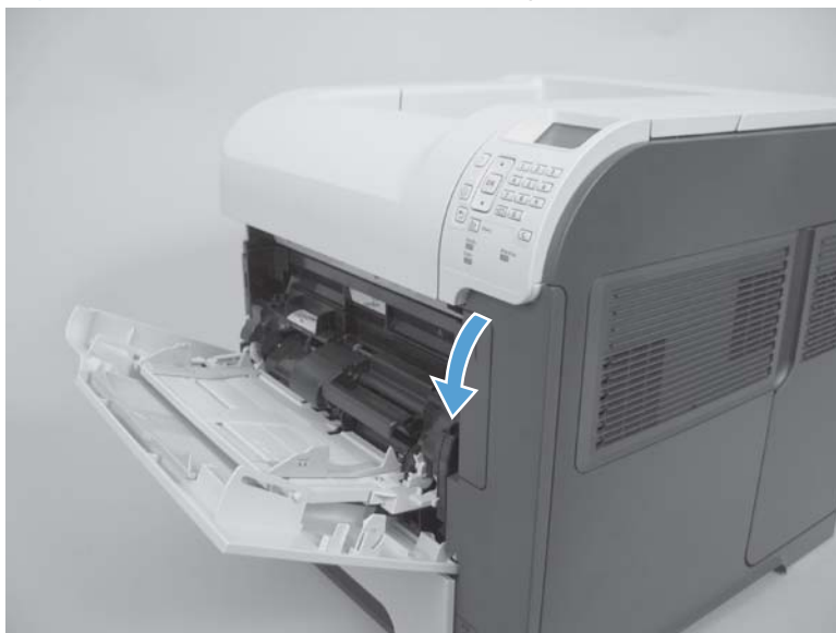
Figure 2-36 Remove the front accessory covers (2 of 2)
