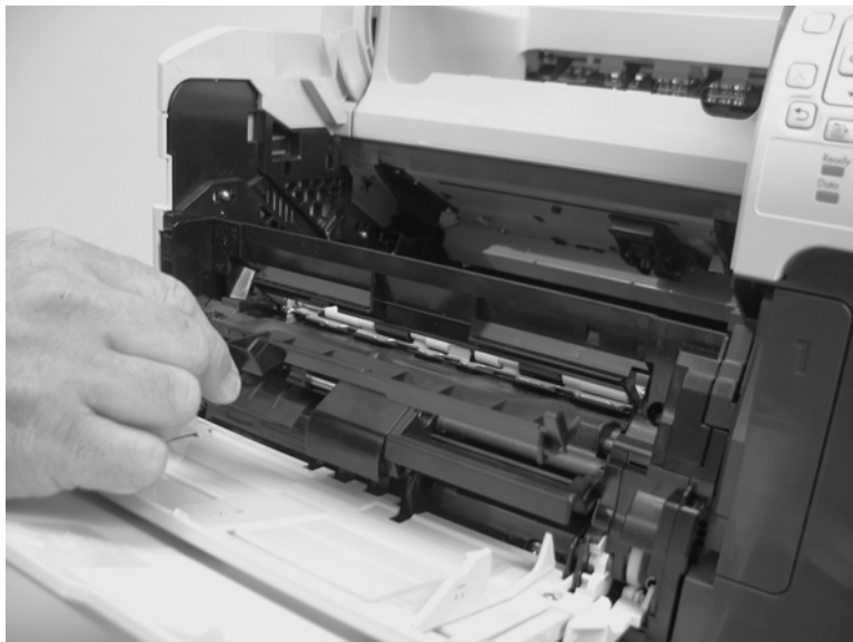
Figure 2-35 Remove the front accessory covers (1 of 2)
