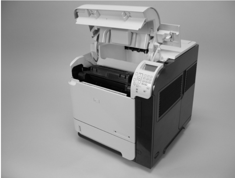
Figure 2-2 Remove the print cartridge (1 of 2)
