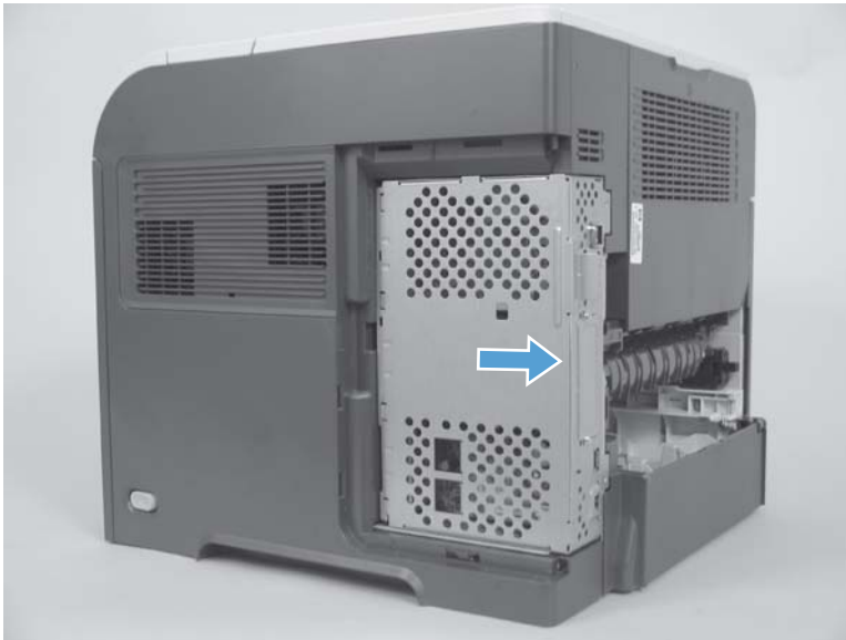
Figure 2-14 Remove the formatter cover and formatter cage (3 of 3)
