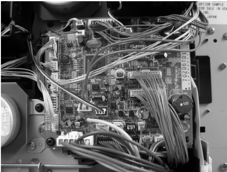
Figure 2-87 Remove the DC controller PCA (1 of 4)
