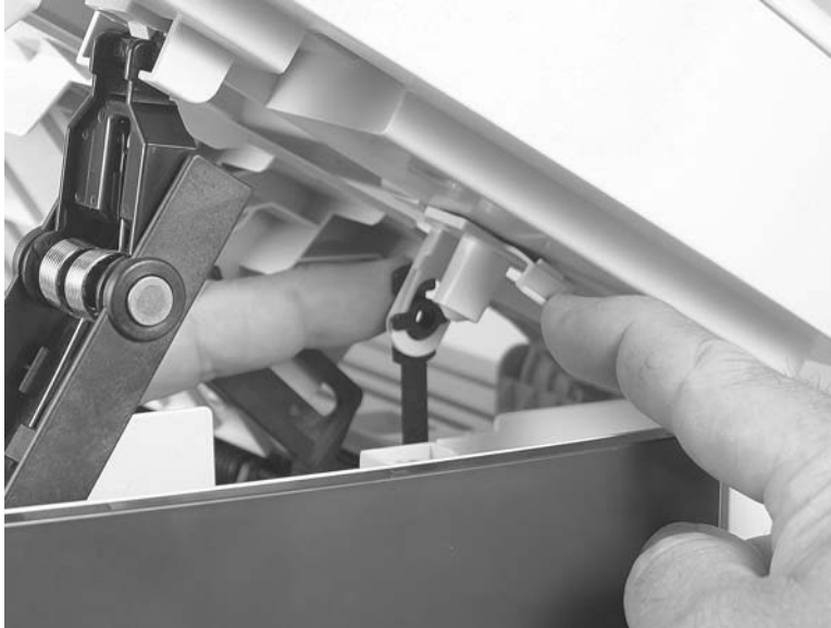
Figure 5-19 Remove the scanner assembly (7 of 10)
