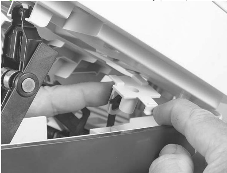
Figure 5-20 Remove the scanner assembly (8 of 10)
