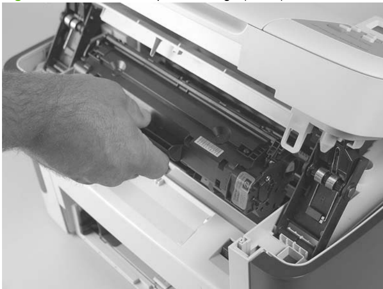
Figure 5-24 Remove the print cartridge (2 of 2)
