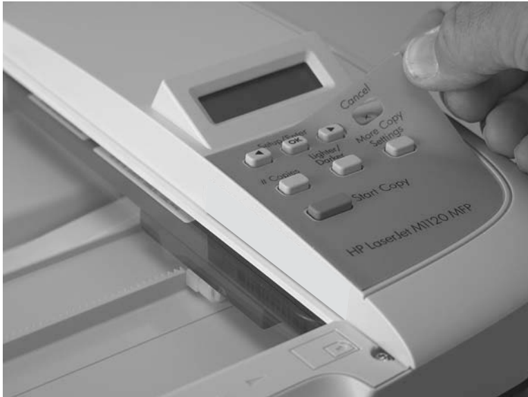
Figure 5-9 Remove the control-panel overlay
