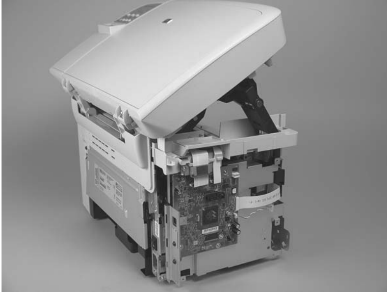
Figure 5-17 Remove the scanner assembly (5 of 10)
