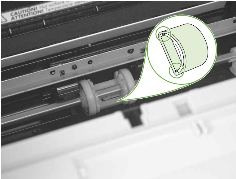
Figure 5-30 Remove the pickup roller (4 of 5)
