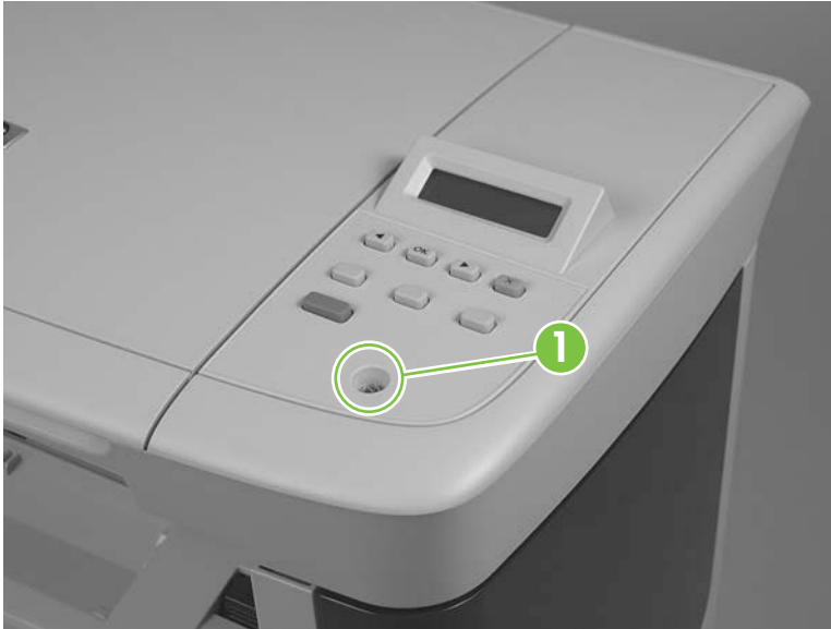
Figure 5-10 Remove the control-panel assembly (1 of 3)
