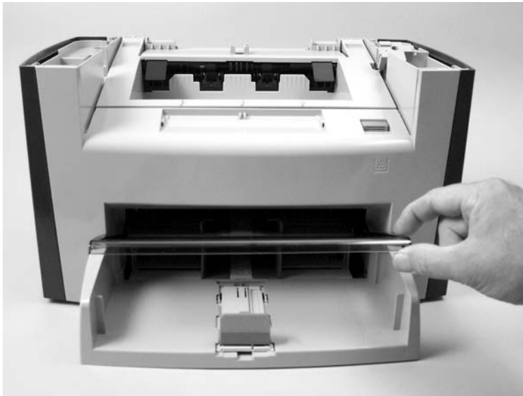
Figure 5-33 Remove the media input tray (1 of 3)
