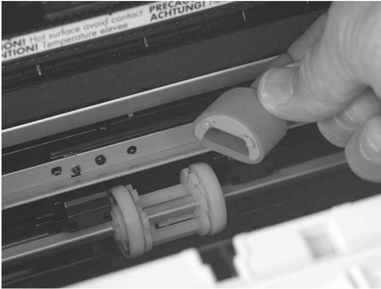
Figure 5-29 Remove the pickup roller (3 of 5)
