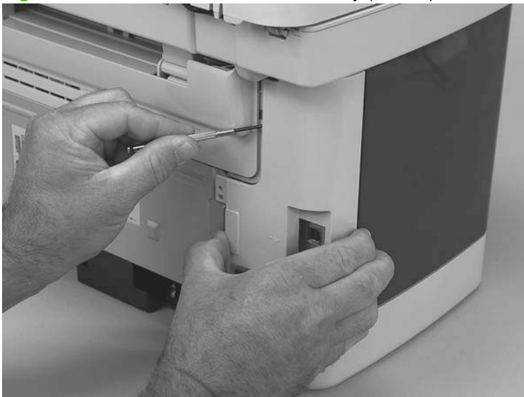
Figure 5-14 Remove the scanner assembly (2 of 10)
