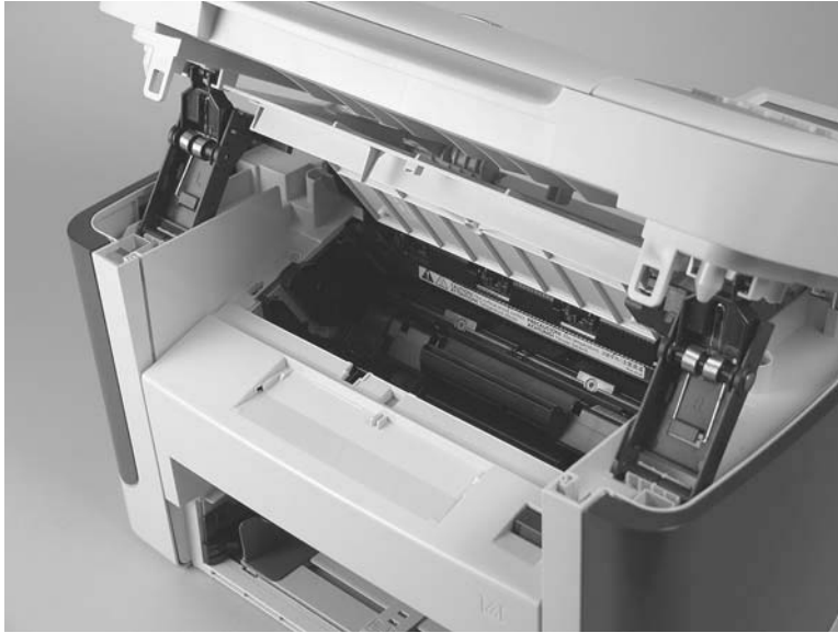
Figure 5-23 Remove the print cartridge (1 of 2)
