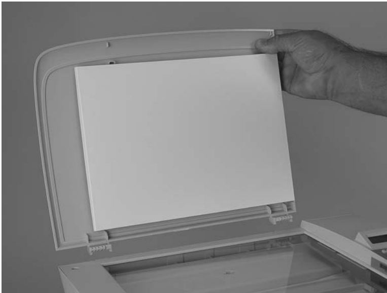
Figure 5-8 Remove the scanner lid (2 of 2)
