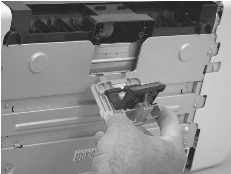
Figure 5-26 Remove the separation pad (2 of 2)
