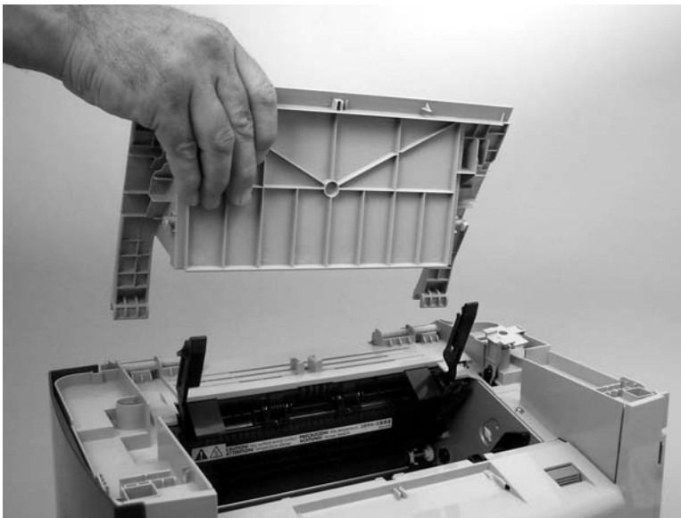
Figure 5-42 Remove the print-cartridge door (2 of 2)
