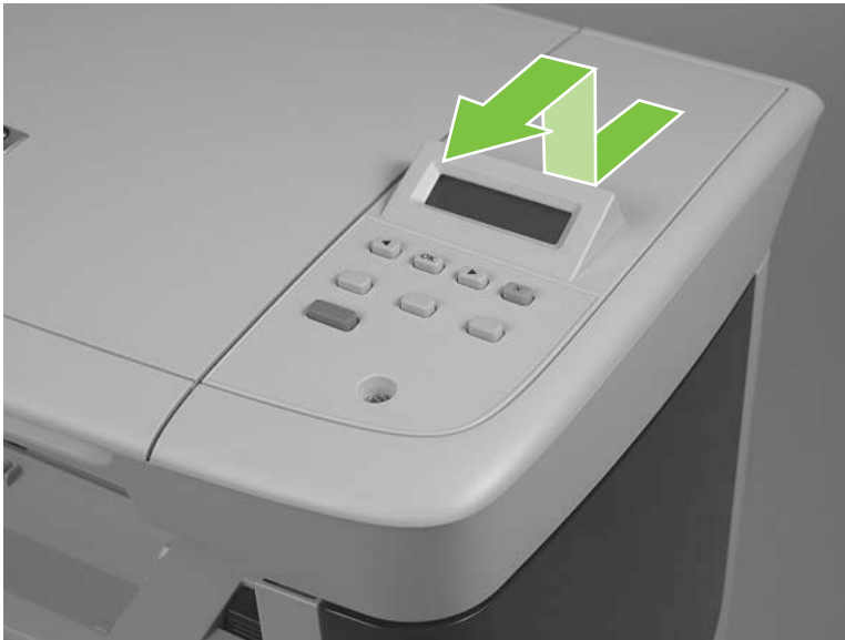
Figure 5-11 Remove the control-panel assembly (2 of 3)
