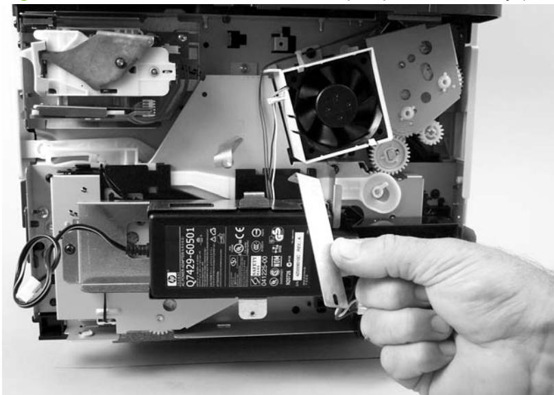
Figure 5-45 Remove the convenience-stapler power assembly (2 of 3)
