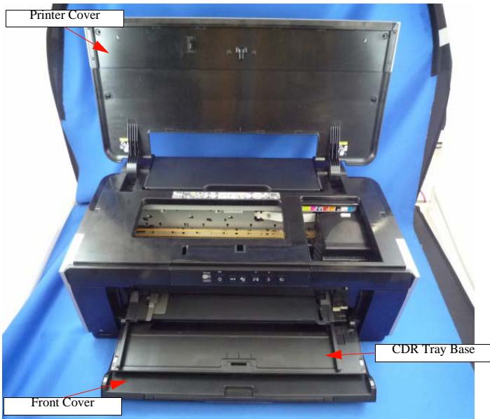
Figure 8-3. Removing the Panel FFC Cover (1)
