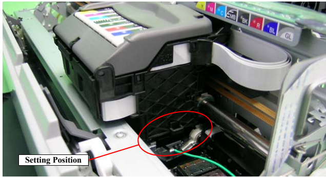
Figure 5-11. Moving the Carriage Unit
