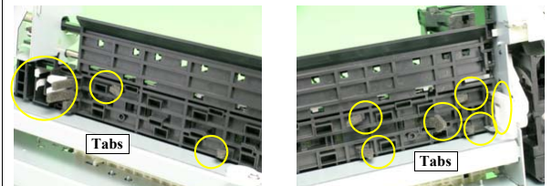
Figure 4-99. Reinstalling the Front Paper Guide Pad (1)
