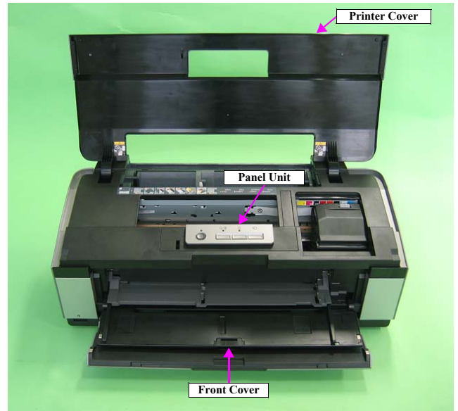
Figure 4-13. Removing the Panel Unit (1)
