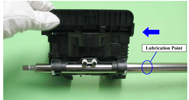
Figure 6-17. Lubricating the Carriage Shaft (4)
